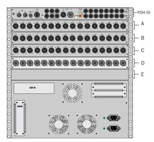
Figure 2-29 Mix Rack back panel slots A-E
