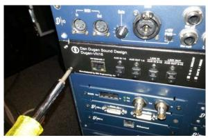
Figure 2-24 Securing the Dugan-VN16 card to the back panel of the FOH Rack
