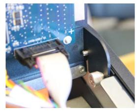
Figure 2-3 Correct alignment of Top Panel slot and pivot post
