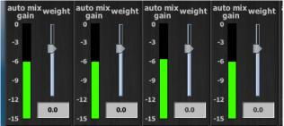
Figure 4-10 Multiple mic ambience: auto mix gain hovers around -9 dB for eight mics, -6 dB for four mics
