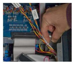
Figure 2-6 Loosening the output card captive thumbscrew
