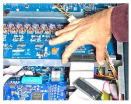
Figure 2-7 Disconnecting ribbon cable from the output card in slot D
