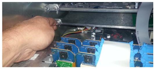
Figure 2-31 Securing the Dugan-VN16 card to its mounting brackets
