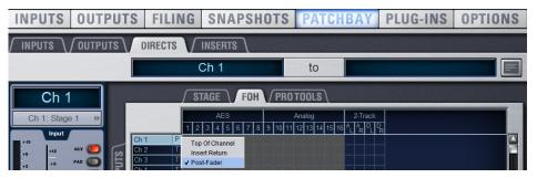
Figure 3-3 Setting the channel Post Fader
