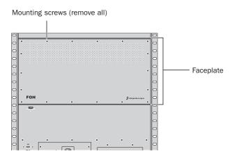
Figure 2-18 Front panel of the FOH Rack
