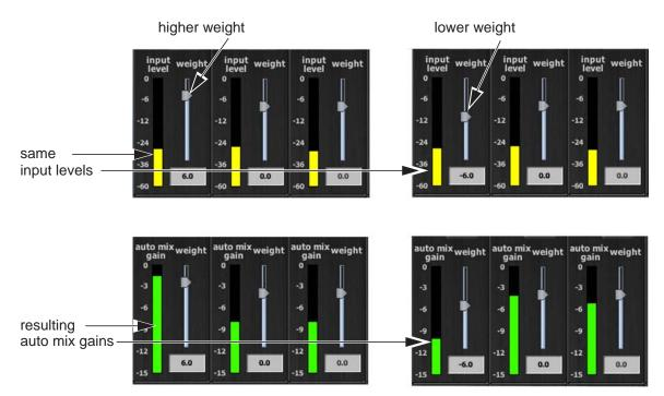
Figure 4-9 Changing one channel's weight control
