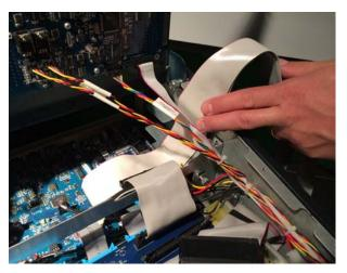
Figure 2-11 Routing the ribbon cables next to the chassis wall (viewed from right side of SC48)
