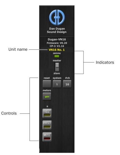
Figure 4-11 Master Pane indicators and controls
