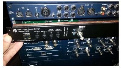
Figure 2-22 Installing the Dugan-VN16 card in the FOH Rack
