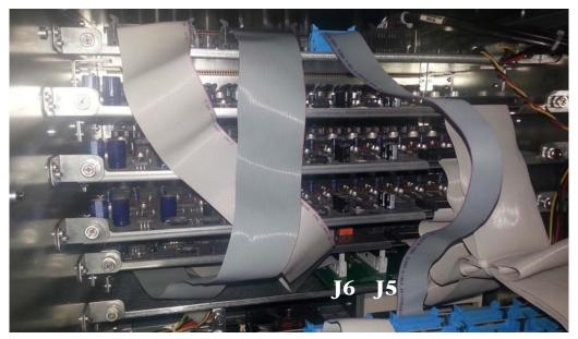
Figure 2-32 Dugan-VN16 ribbon cables connected to FOH IO card
