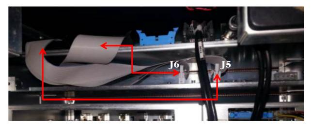
Figure 2-25 Ribbon cables connecting the Dugan-VN16 card to the I/O card
