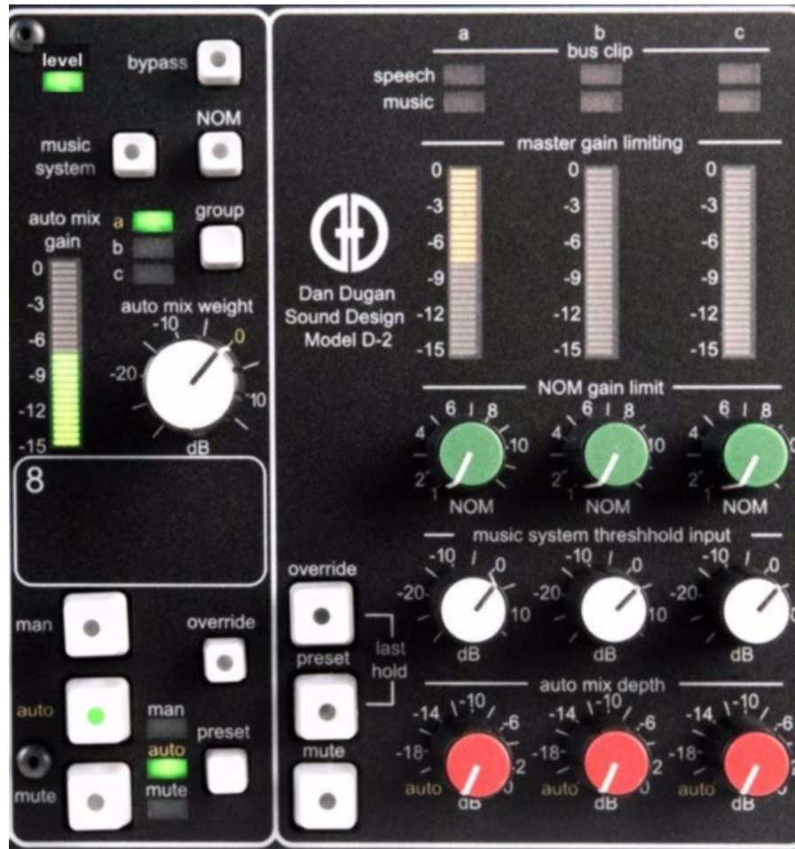
Figure 3-2 Channel and Master sections
