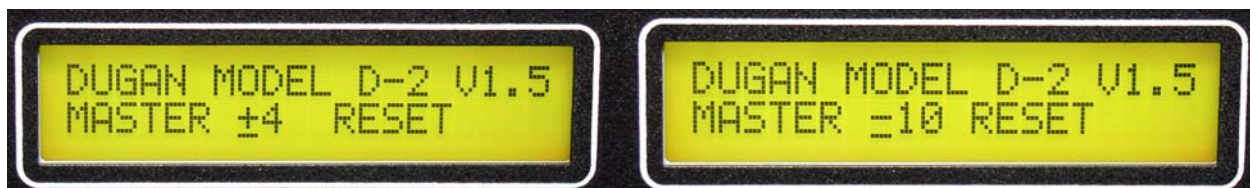
Q-9 Changing the level mode from +4 to -10
