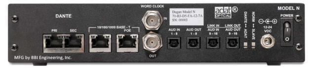
Figure 3-1 Model N rear panel connectors
