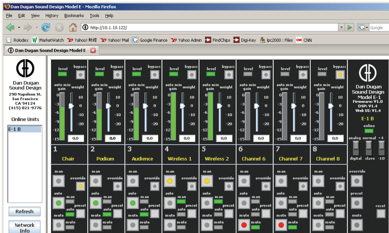
An internal Web server downloads a Java applet that provides a real-time remote control panel in any Web browser
