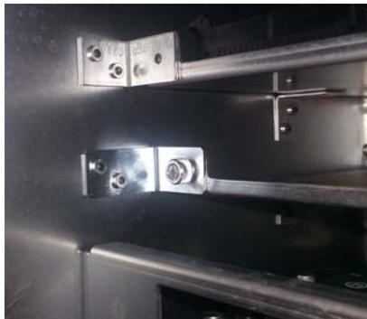
**Figure 2-23** Securing a card to the mounting brackets
