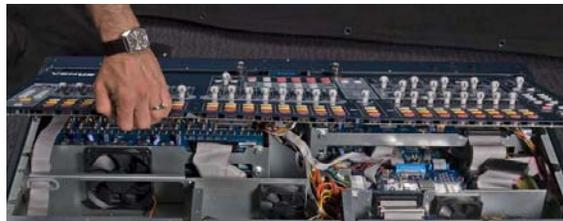
**Figure 2-2** Lifting the Top Panel to vertical
