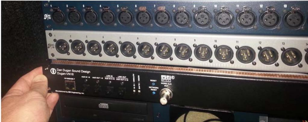
**Figure 2-30** Sliding the Dugan-VN16 card into Slot E
