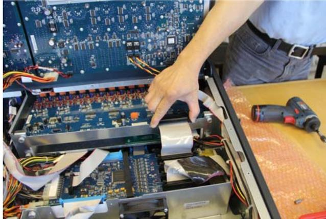
**Figure 2-16** Reconnecting the ribbon cable on the output card
