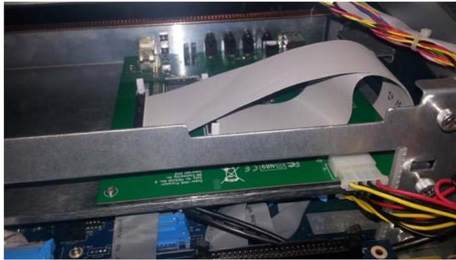
**Figure 2-15** Connecting an available power cable to the Dugan-VN16 card
