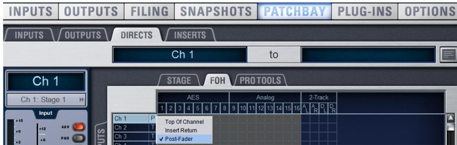
Figure 3-3 Setting the channel Post Fader
