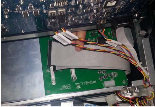
**Figure 2-13** Installing a card into slot E
