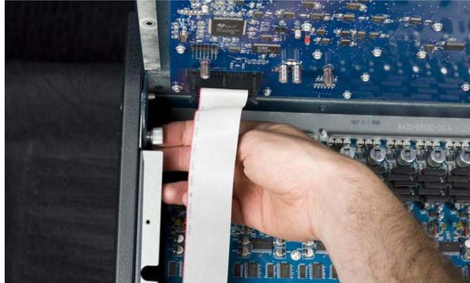
**Figure 2-4** Tightening the top left captive thumbscrew
