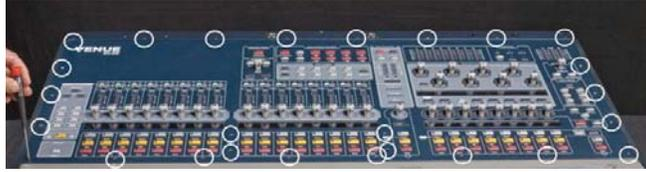
**Figure 2-1** Removing the 26 Top Panel screws
