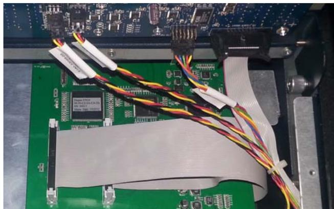
**Figure 2-14** Connecting ribbon cables to the Dugan-VN16 card
