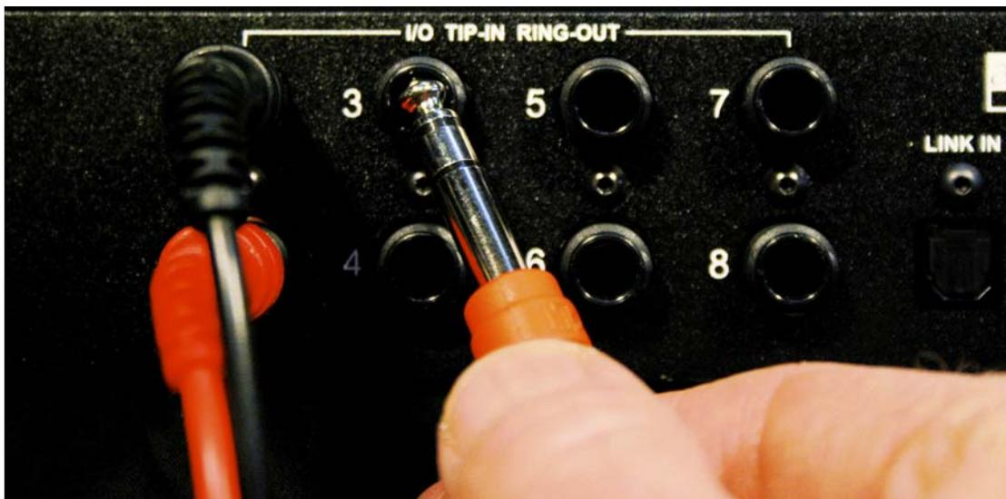
Figure 2-1 Analog connection
