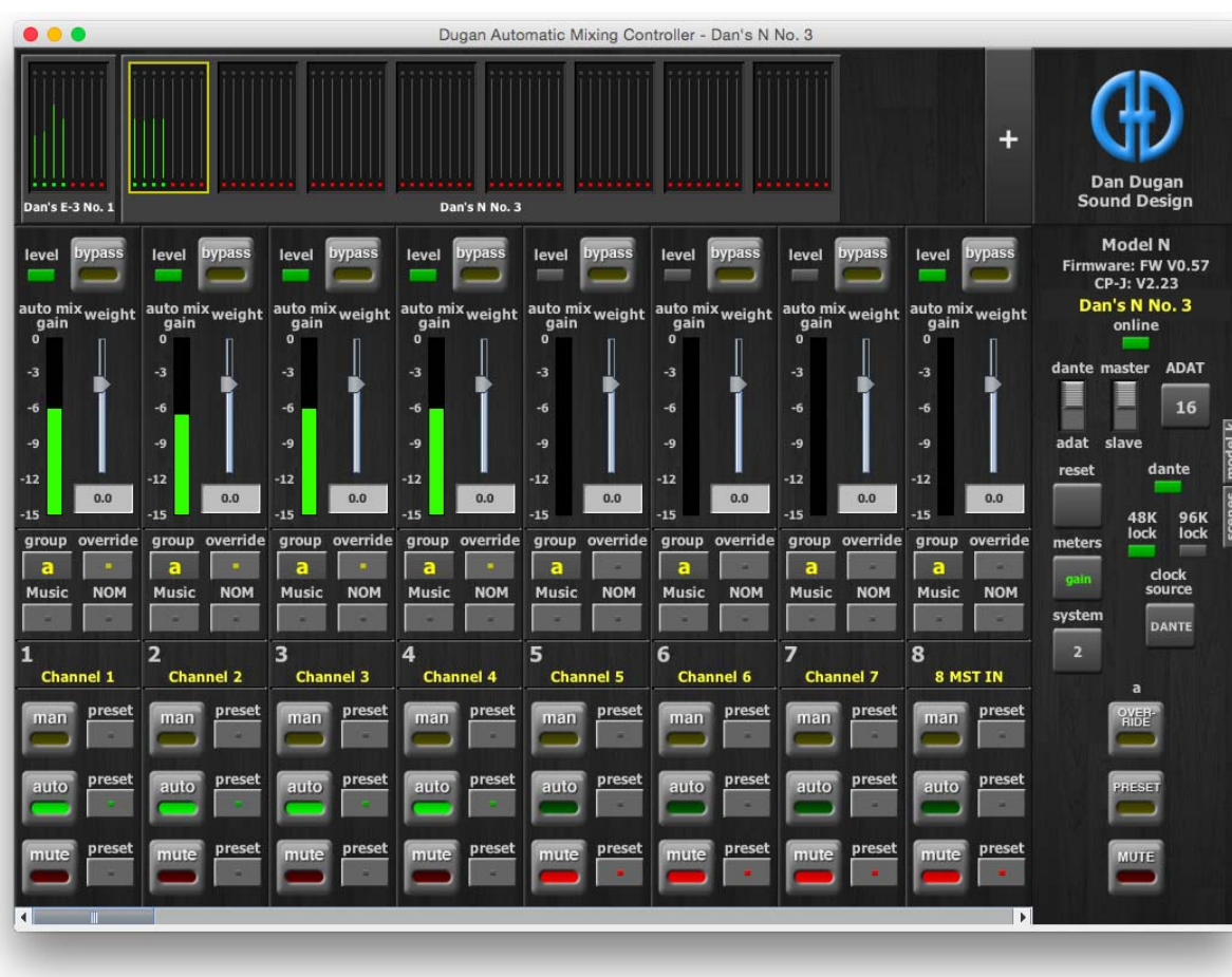
Figure 5-1 Dugan Control Panel
